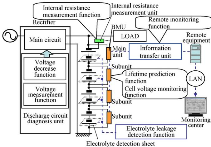
Fig. 4. Configuration of system for remote management of VRLA batteries.
