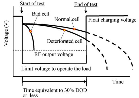
Fig. 7. Outline of discharge circuit diagnosis function.
