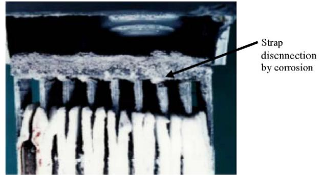
Fig. 3. VRLA battery strap corrosion.
