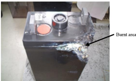
Fig. 2. VRLA battery burnt by electrolyte leakage.
