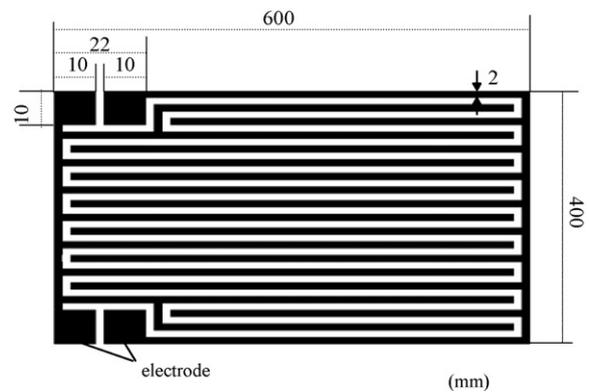
Fig. 8. Copper-foil electrode pattern in detection sheet.
