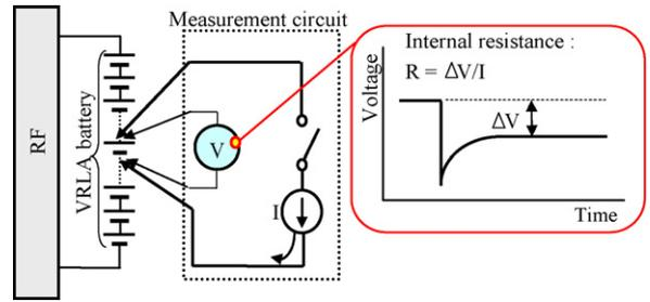
Fig. 11. Circuit for measuring internal resistance with short time discharge method.
