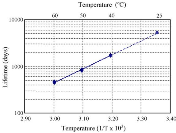
Fig. 6. Correlation between battery lifetime and ambient temperature.
