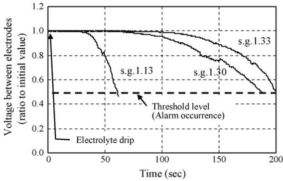
Fig. 10. Electrolyte leakage detection by electrolyte leakage detection unit.
