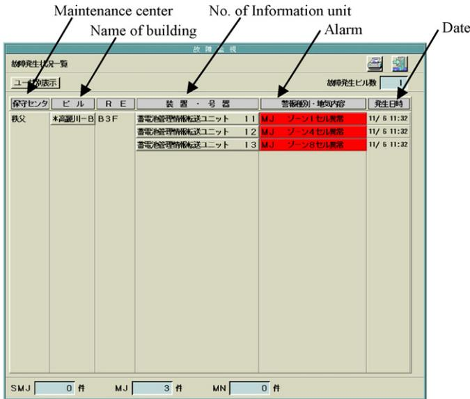
Fig. 13. Example of monitoring center displaying cell malfunction.
