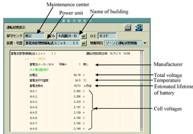
Fig. 14. Example of monitoring center displaying battery status.
