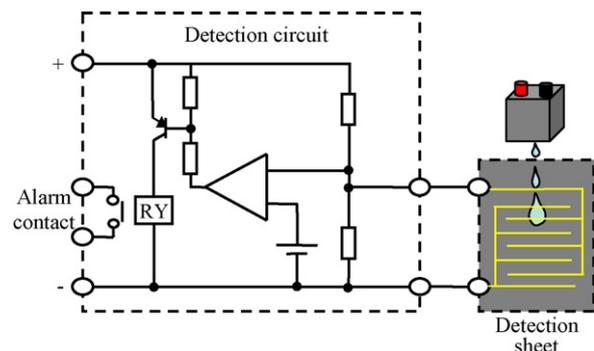
Fig. 9. Electrolyte leakage detection circuit diagram.
